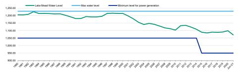
Improvements have been made such that the minimum level of Lake Mead elevation for power generation has been reduced to 950 feet, from the previous 1,050 foot level
